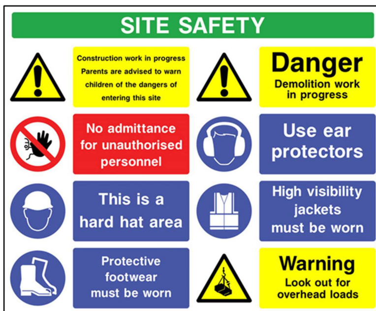
Figure 5-1 - Example of Site Safety Signage
